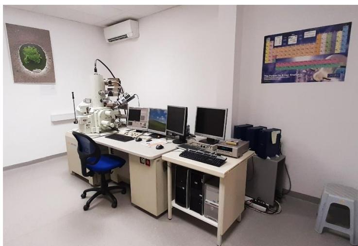
*Figure 2. Scanning electron microscope JSM-7600F.*
