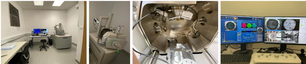
*Figure 4. Scanning electron microscope ESEM Quanta 650.*
