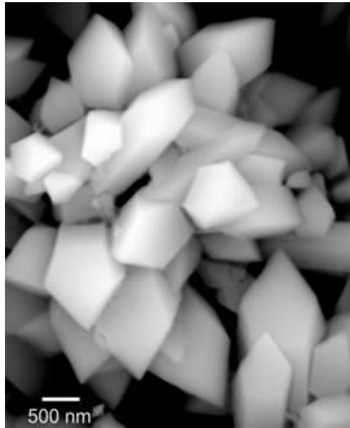
Slika 7. Kristali (\text{Nd,Na})(\text{SO}_4)_2 \times \text{H}_2\text{O} . (Xu. X., Samardžija Z., K7, JSM 7600F).
