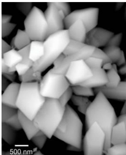
Figure 7. (Nd,Na)(SO 4 ) 2 x H 2 O crystals (Xu. X., Samardžija Z., K7, JSM 7600F).
