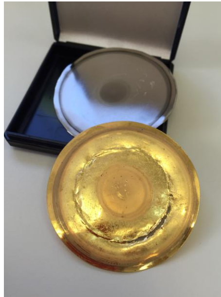
Magnetron target (Au, Pt) demonstrating racetrack erosion profile
